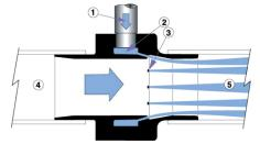
Compressed air flows through the inlet (1) into an annular plenum chamber (2). It is then injected into the throat through directed nozzles (3). These jets of air create a vacuum at the intake (4) which draws material in and accelerates it through the unit (5) for conveying over long vertical or horizontal distances.
