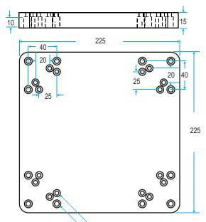
Countersunk holes for use with M5 cap screws (x16) Countersunk holes for use with M6 cap screws (x12)
